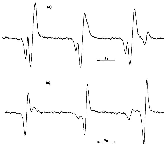
FIG. 3 ESR spectra of nitroxide radicals formed during photolysis of benzophenone in the presence of di-isopropyl sulphide and t -nitrosobutane. (a) Spectrum observed during photolysis, (b) spectrum observed directly after photolysis.
